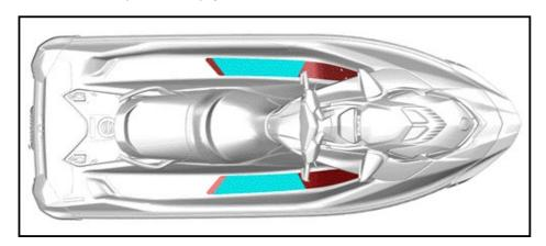
4. Using footrests, make marks on deck and drill marks using a 5.5 mm (7/32 in) drill bit.
