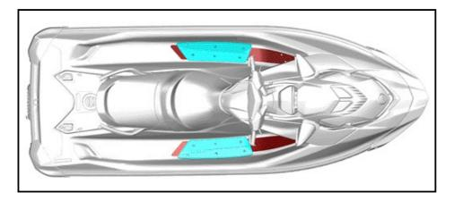
2. Mark both original anti-slip mats as per footrests location with an extra 6 mm (1/4 in) to the back and front section of the footrest length.
