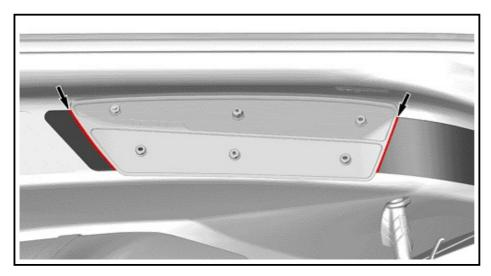
3. Remove the marked sections of the anti-slip mats located under the footrest and only clean the  $6\,$  mm (1/4 in) front and rear section of any excess glue.
